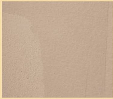
This panel shows the touchup on a competitive latex flat. Despite correct application procedures, the touchup is clearly visible.
